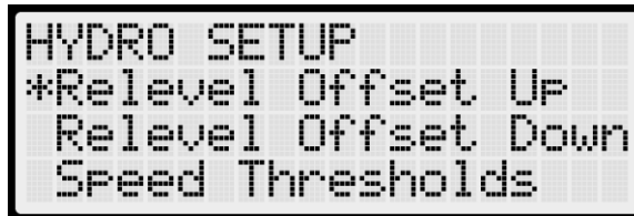
Figure 331: HYDRO SETUP Menu – Relevel Offset, Speed Thresholds
