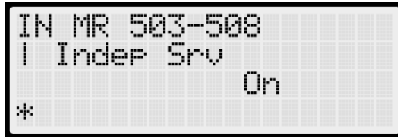
Figure 199: Invert Inputs Menu – Machine Room Example
