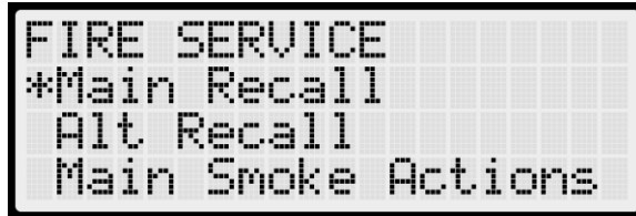
Figure 253: FIRE SERVICE Menu – Main Recall, Alt Recall, Main Smoke Actions
