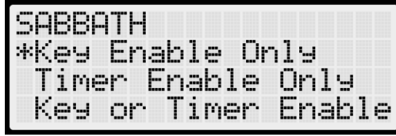
Figure 306: SABBATH Menu – Key Enable Only, Timer Enable Only, Key or Timer Enable
