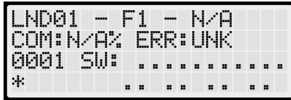
Figure 36: Uninitialized Hall Board Status
